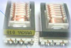
High voltage transformer
