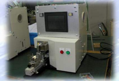
Harness pressure welding / conduction inspection jig
